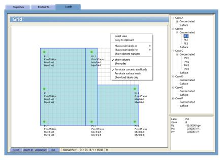
Alternatively, you could have clicked on the Assign button located on the toolbar, and then on the LOADS tab. If columns or piles have been assigned to the model, they are displayed in the color specified for COLUMN or PILES in the DISPLAY SETTINGS. If it is preferred not to show columns or piles, right-click on empty space on the view window, and then uncheck Show Columns or Show Piles on the pop-up menu.
