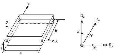
Figure 2-4 Plate Finite Element
