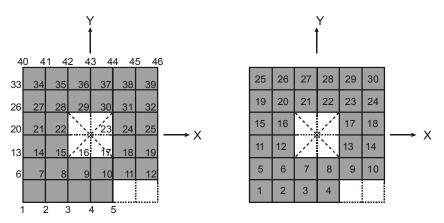
Figure 2-3 Node and Element Numbering
