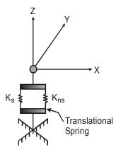
Figure 2-5 Soil Element
