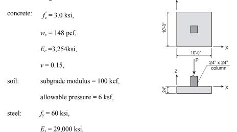
The origin of the XY plane will be located at the lower left-hand corner of the footing. Two-foot square elements will be used; thus, the grid system consists of six grid lines (i.e. five elements), two feet apart, in each direction. The concentrated load will be applied as four nodal loads (125 kip each). The finite element mesh is shown at the end of this example.
